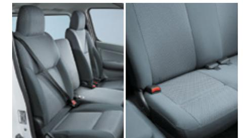
The driver and front seat passenger seats are equipped with seatbelts featuring pretensioners and load limiters. In minibus models, each rear passenger seat features 2-point seatbelts.
